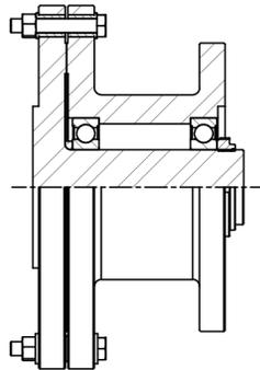
Shear Pin Coupling
